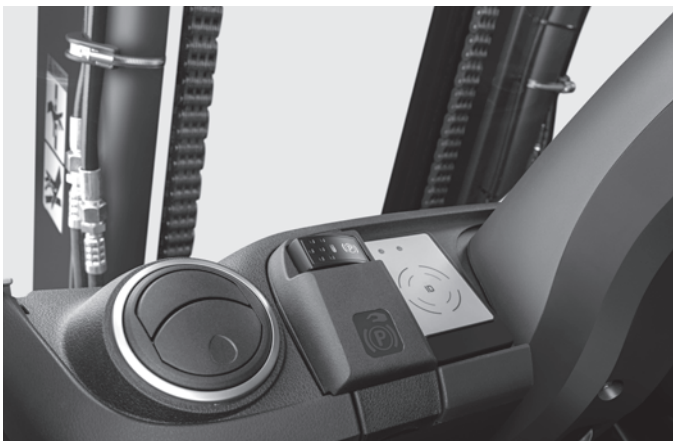
Perfect stability in every position thanks to the electro-hydraulic parking brake
